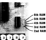
The first chip in the stack is enabled The Inst chip in the stack is enabled via the Expansion Port socket wiring. The other chips are enabled by connecting a jumper lead from pin 18 to one of the pins as shown above.
