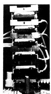
Two 'units' piggy-backed together. The lower chip is accessed via the PC board; the top chip via the jumper lead.
